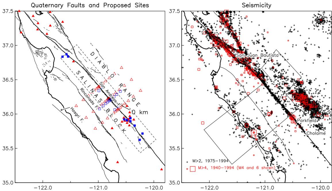
Figure 1. On the left, red triangles are CGPS, and blue squares borehole strain: in both cases, solid for existing or planned, open for proposed here.
