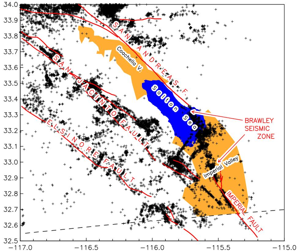
Figure 1. Major faults and seismicity in and around the Salton Trough. Epicenters from the relocation by Richards-Dinger and Shearer.
