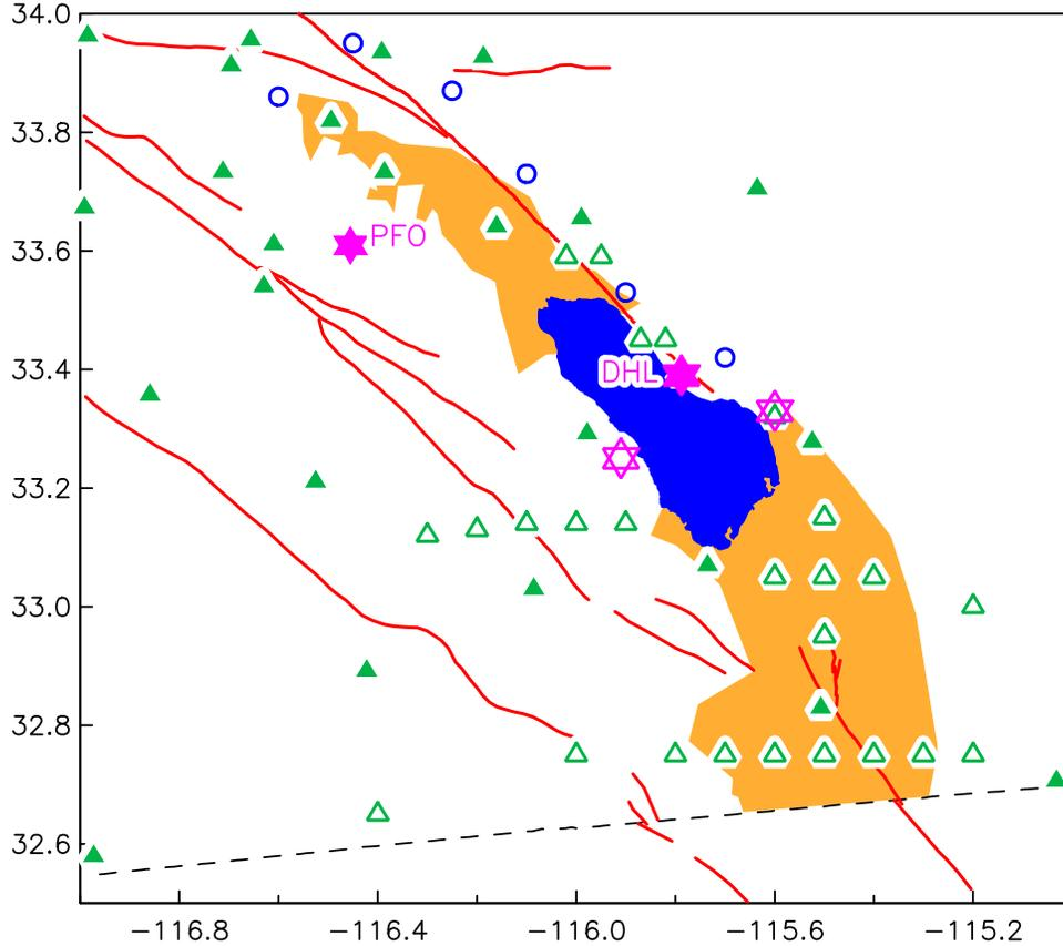
Figure 2. Existing (solid) and proposed (open) deformation measurements in the Salton Trough. Continuous GPS is green triangles, long-base strain purple stars, borehole strain blue circles.
