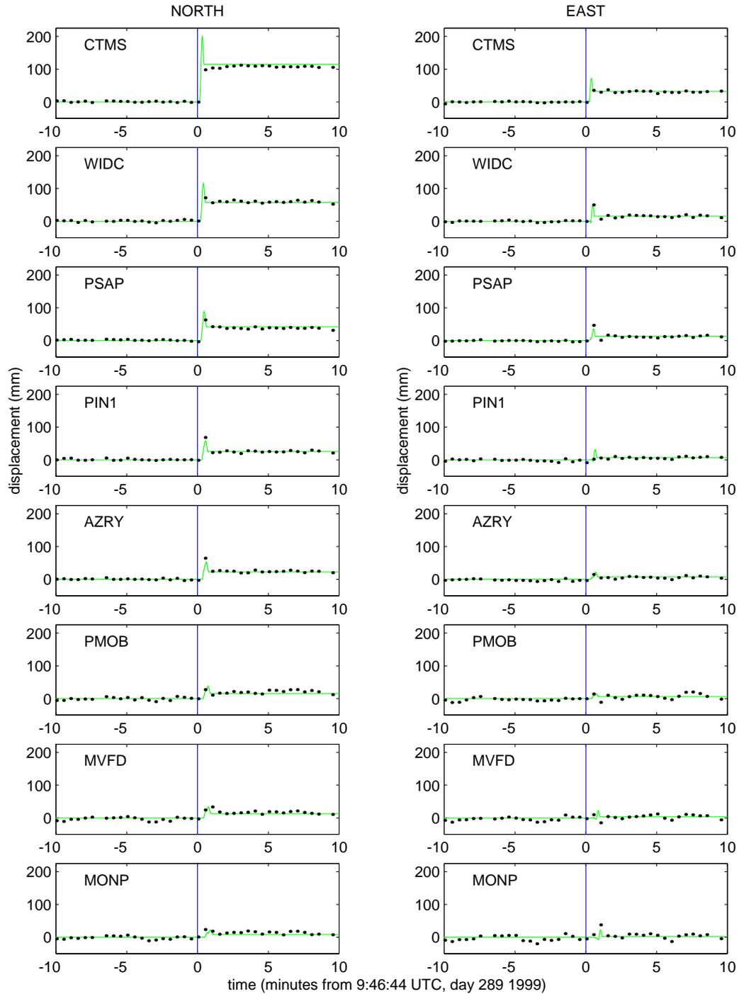
**Figure 3.** Observed horizontal displacements along a north-south profile of SCIGN stations within 10 minutes of the October 16, 1999 Hector Mine earthquake (blue line). Data are sampled at 30 s. Sites are in order of closest (top) to farthest (bottom) from the epicenter. The gray line shows model displacements based on a double couple source in a homogeneous elastic whole space.
