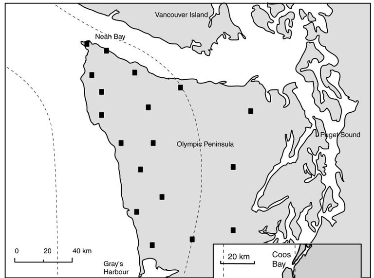
**Figure 2** Preliminary design of the borehole strainmeter + tiltmeter arrays on the Olympic peninsula (18 sites) and Cape Blanco (4 sites). The dashed lines indicate the position of the transition zone ~10-20km below.
