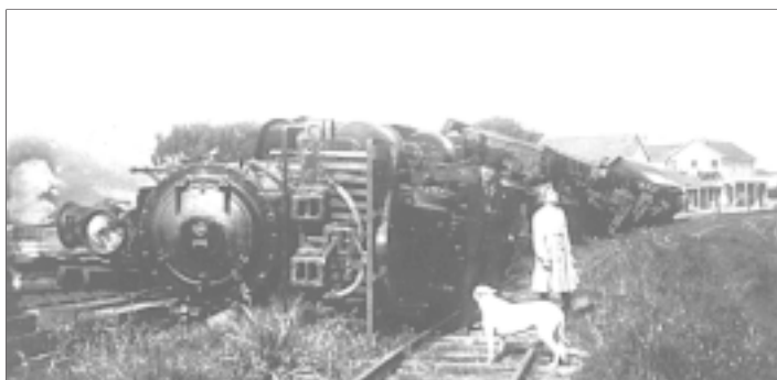
The result of the pulse-like motion that occurs close to a large earthquake can be seen in this photo taken soon after the 1906 earthquake. Thomas Heaton points out that although the pulse motion didn't greatly damage the railroad station in the background, such a motion might have serious consequences for some modern flexible buildings.
