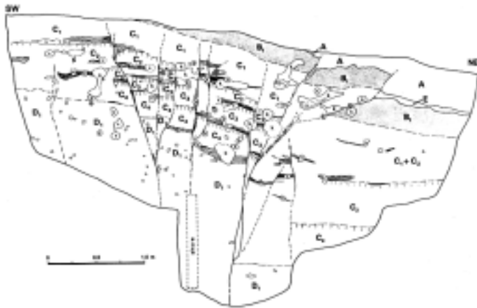
Figure 5. Detailed map of the northwest wall of trench T-4 showing the primary structural elements and stratigraphic units. Unit C was subdivided on the basis of weakly developed buried A horizons (shown as short vertical wavy lines). Unit C contains thin beds and stringers of clay (solid), silt (open), and sand (stippled). Evidence of bioturbation is shown by the numerous krotovina (k). Note that the northeastern strands displace the A, E, and B 1 soil horizons, which is the result of the most recent surface rupture, whereas the southwestern strands could not be traced to the top of unit C 1 .
